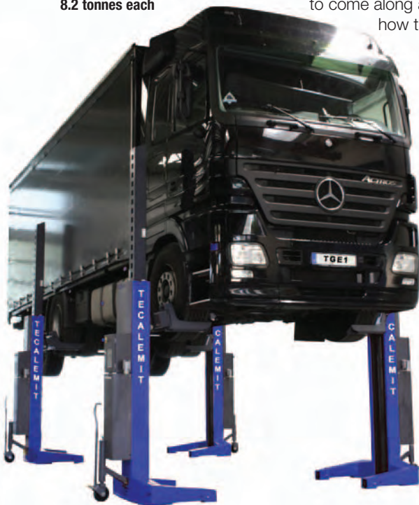
Wireless mobile column lifts from Finkbeiner can lift 8.2 tonnes each
